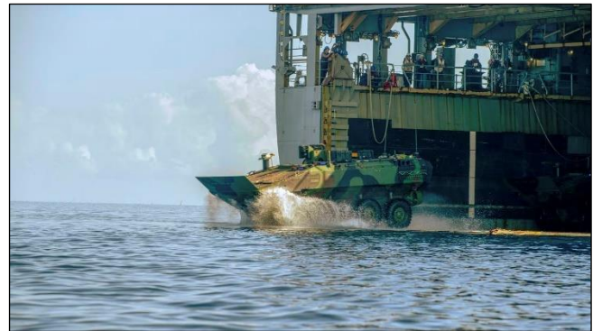
Figure 1. ACV in Ship-to-Shore Mode
