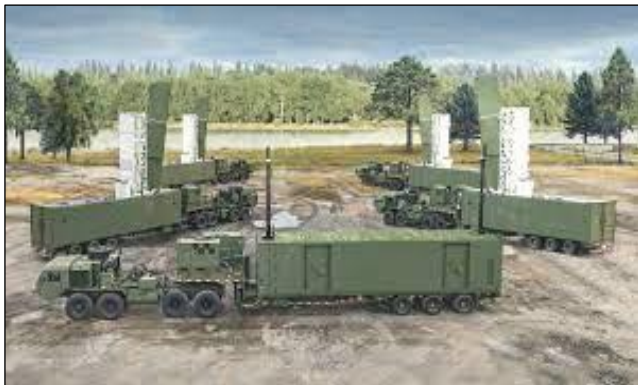
Figure 1. Typhon Launchers and Battery Operations Center
