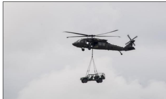
Figure 2. ISV Sling-Loaded Under a UH-60 Helicopter
