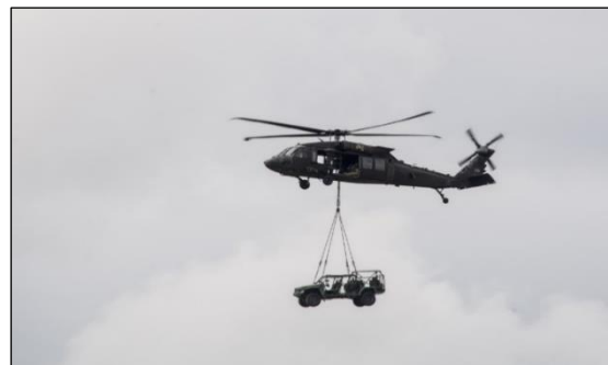
Figure 2. ISV Sling-Loaded Under a UH-60 Helicopter
