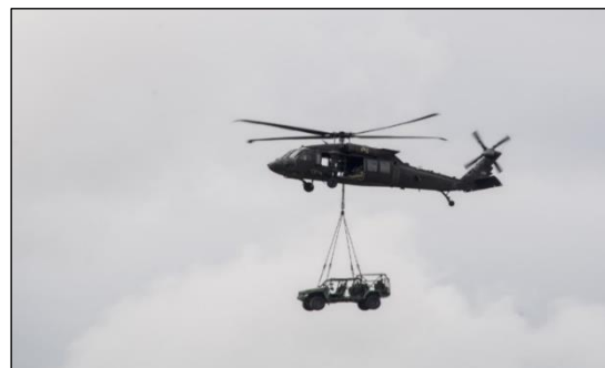
Figure 2. ISV Sling-Loaded Under a UH-60 Helicopter
