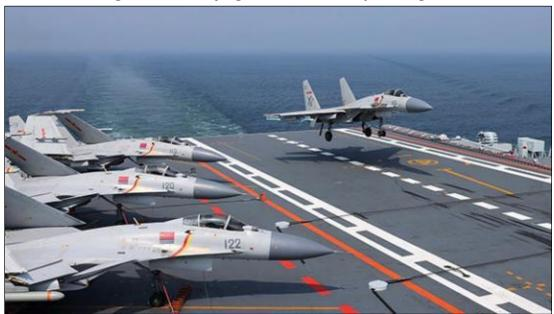
Figure 22. J-15 Flying Shark Carrier-Capable Fighter
