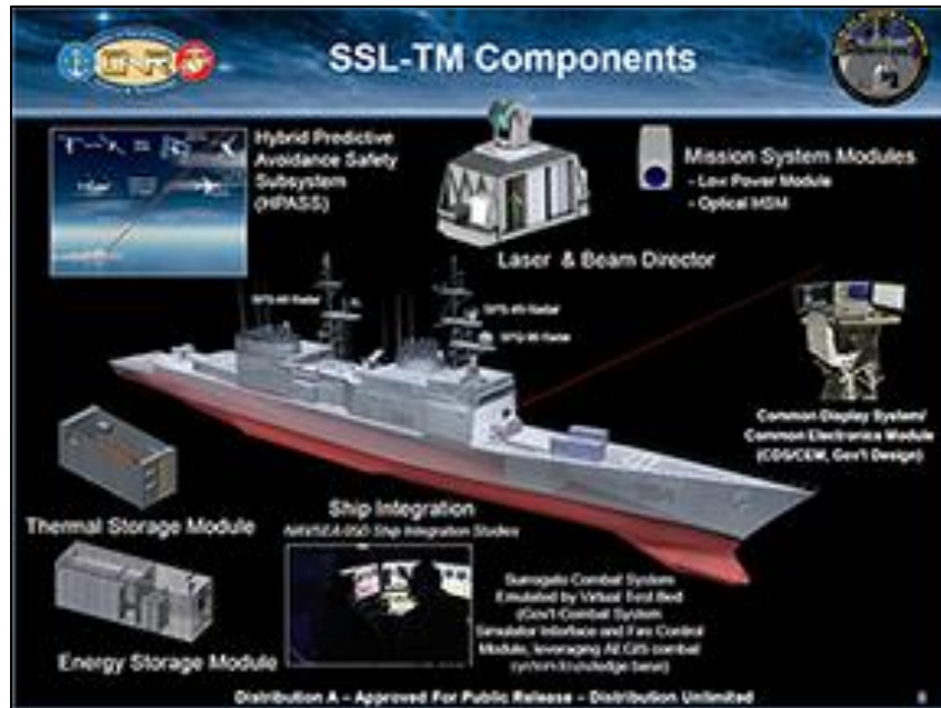
Figure 5. ONR Graphic of SSL-TM Laser System
