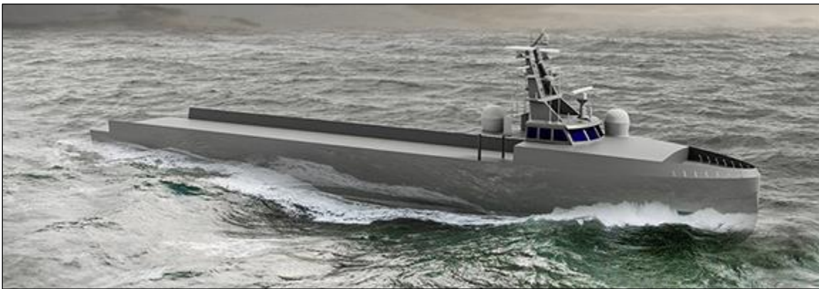
Figure 6. Rendering of L3Harris Design Concept for MUSV
