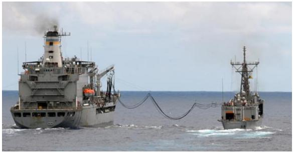
Figure 2. Fleet Oiler Conducting an UNREP
