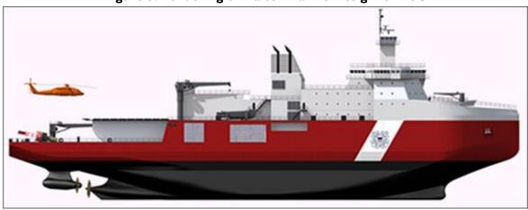
Figure 3. Rendering of Halter Marine Design for PSC
