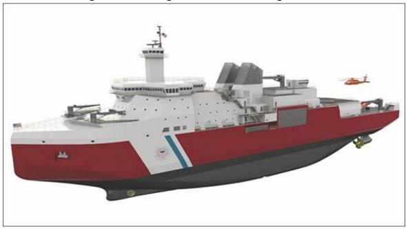
Figure 1. Rendering of Halter Marine Design for PSC
