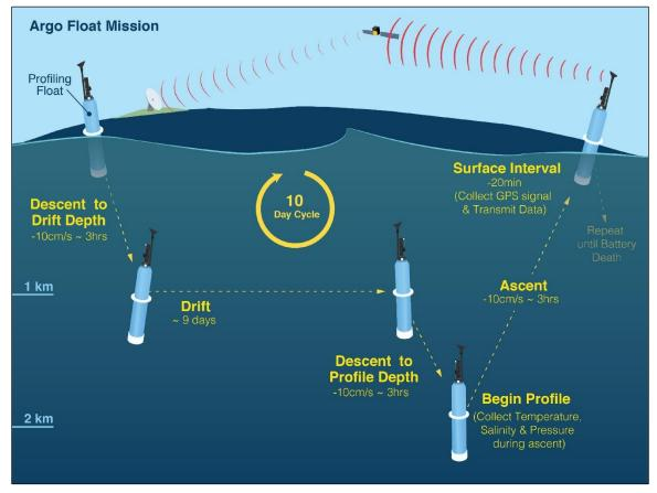
Figure I. NOAA Argo Profiling Float 10-Day Data Collection Cycle
