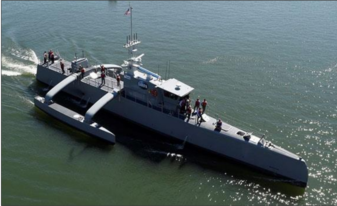
Figure 2. Sea Hunter Prototype Medium Displacement USV
