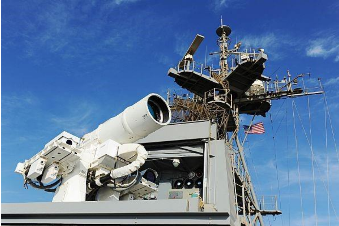
Figure 1. Laser Weapon System (LaWS) on USS Ponce
