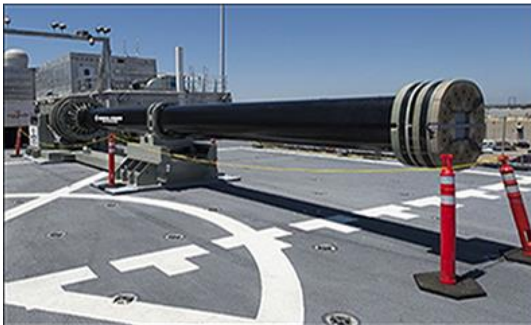
Figure 15. Industry-Built EMRG Prototype Demonstrator
