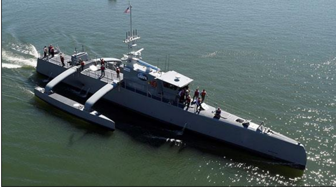
Figure 4. Sea Hunter Prototype Medium Displacement USV
