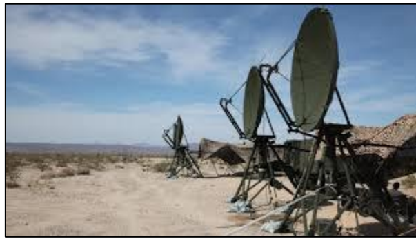
Figure 4. AN/TRC-170 Tropospheric Scatter Microwave Radio Terminal
