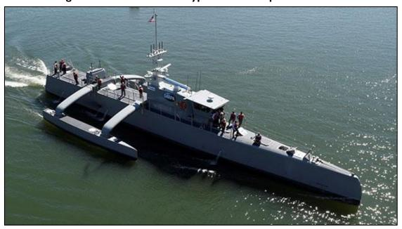
Figure 4. Sea Hunter Prototype Medium Displacement USV
