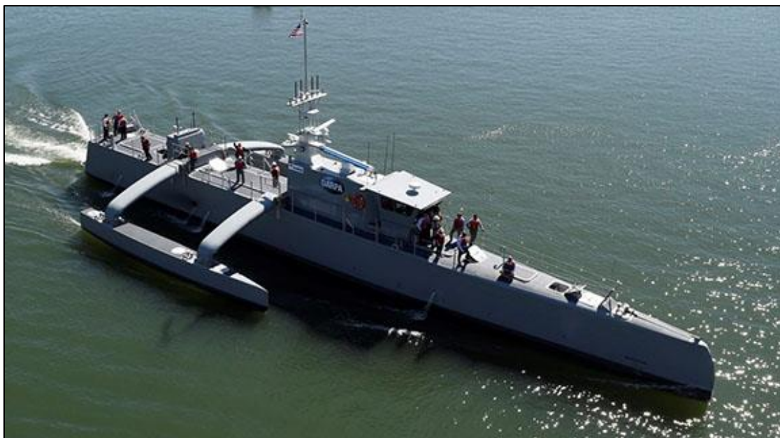
Figure 4. Sea Hunter Prototype Medium Displacement USV
