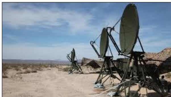
Figure 4. AN/TRC-170 Tropospheric Scatter Microwave Radio Terminal
