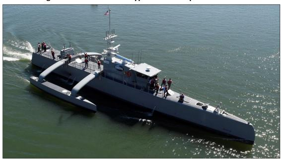
Figure 5. Sea Hunter Prototype Medium Displacement USV
