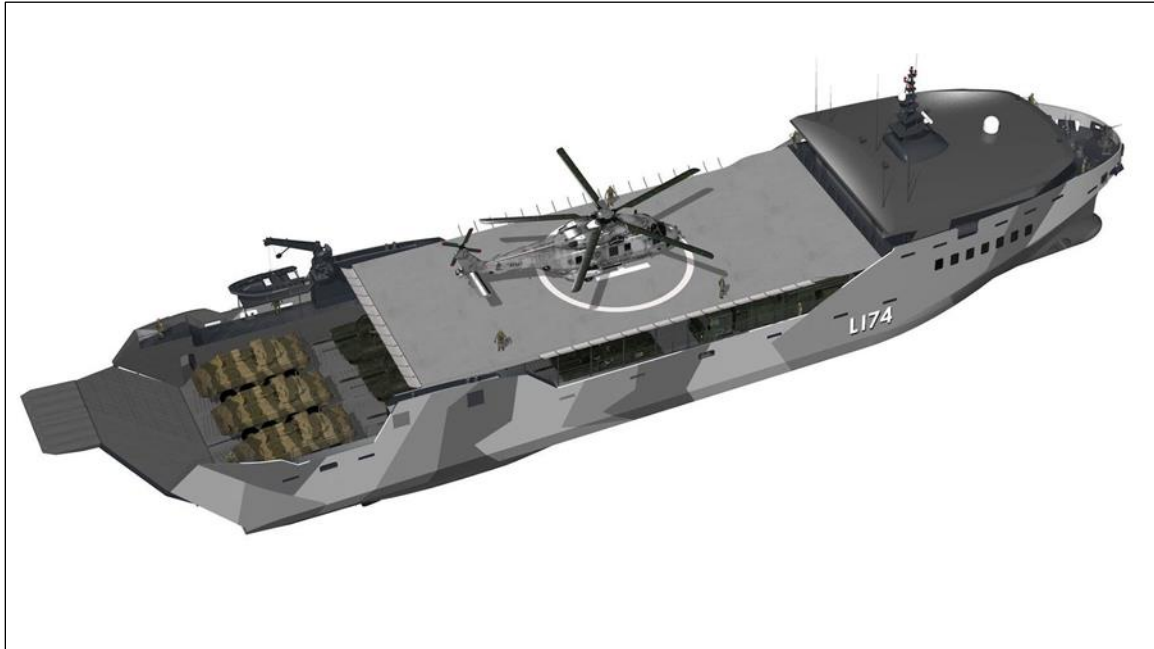
Figure 3. Notional Design for a LAW-Like Ship
