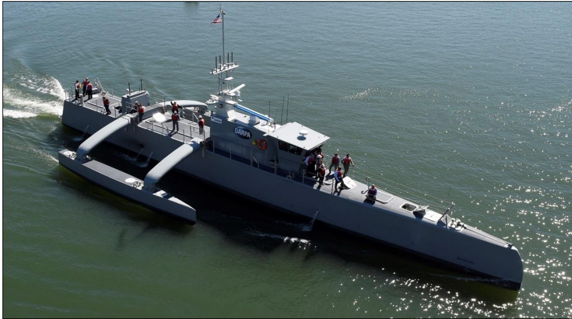
Figure 5. Sea Hunter Prototype Medium Displacement USV
