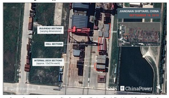
Figure 11. Type 002 Aircraft Carrier Under Construction
