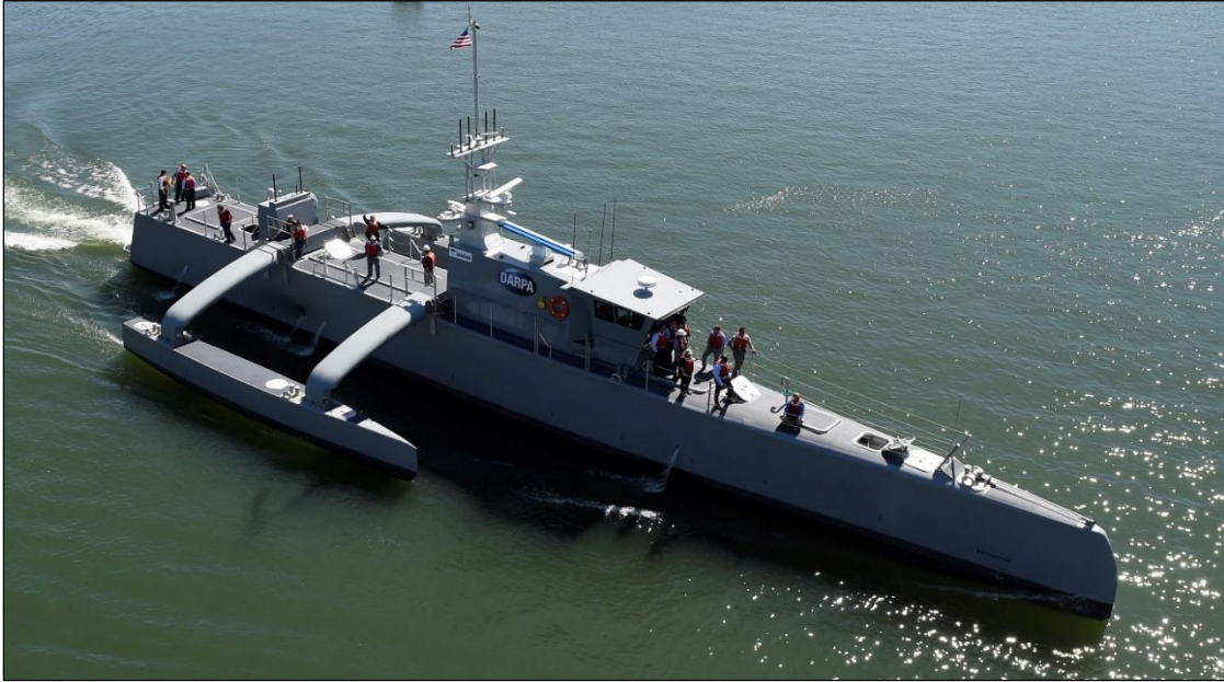
Figure 5. Sea Hunter Prototype Medium Displacement USV
