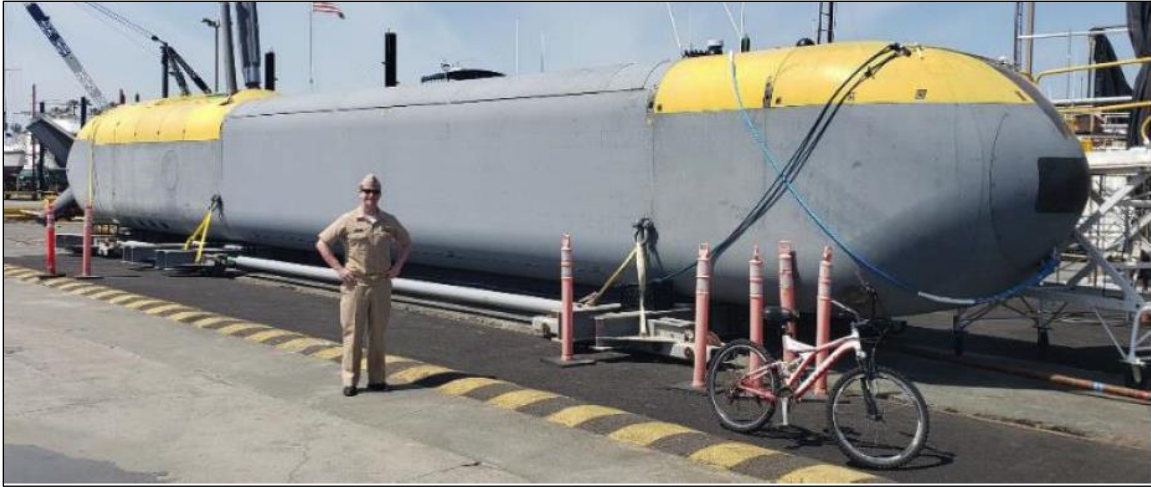
Figure 9. Boeing Echo Voyager UUV
