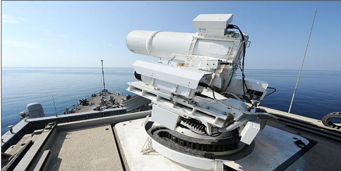
Figure 2. Laser Weapon System (LaWS) on USS Ponce
