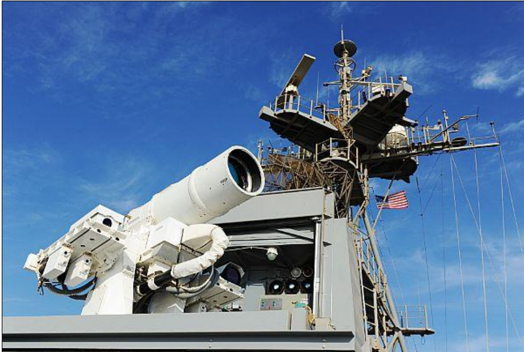
Figure 1. Laser Weapon System (LaWS) on USS Ponce
