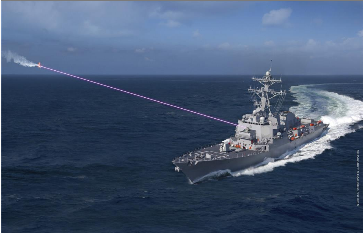
Figure 5. HELIOS System on DDG-51 Destroyer Artist's rendering
