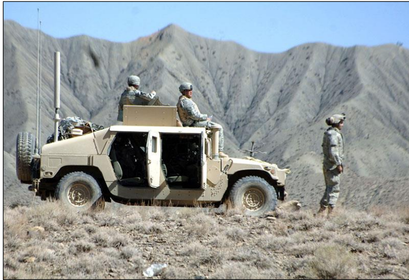
Figure 3. Duke Version 3 Vehicle Mounted CREW system
