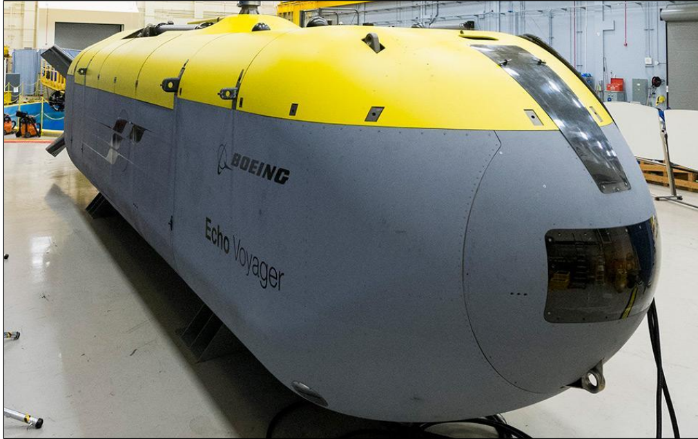
Figure 8. Boeing Echo Voyager UUV
