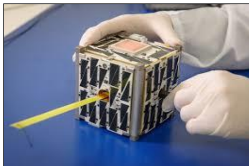
Figure 1. Cubesat Constructed from Smartphone Parts
