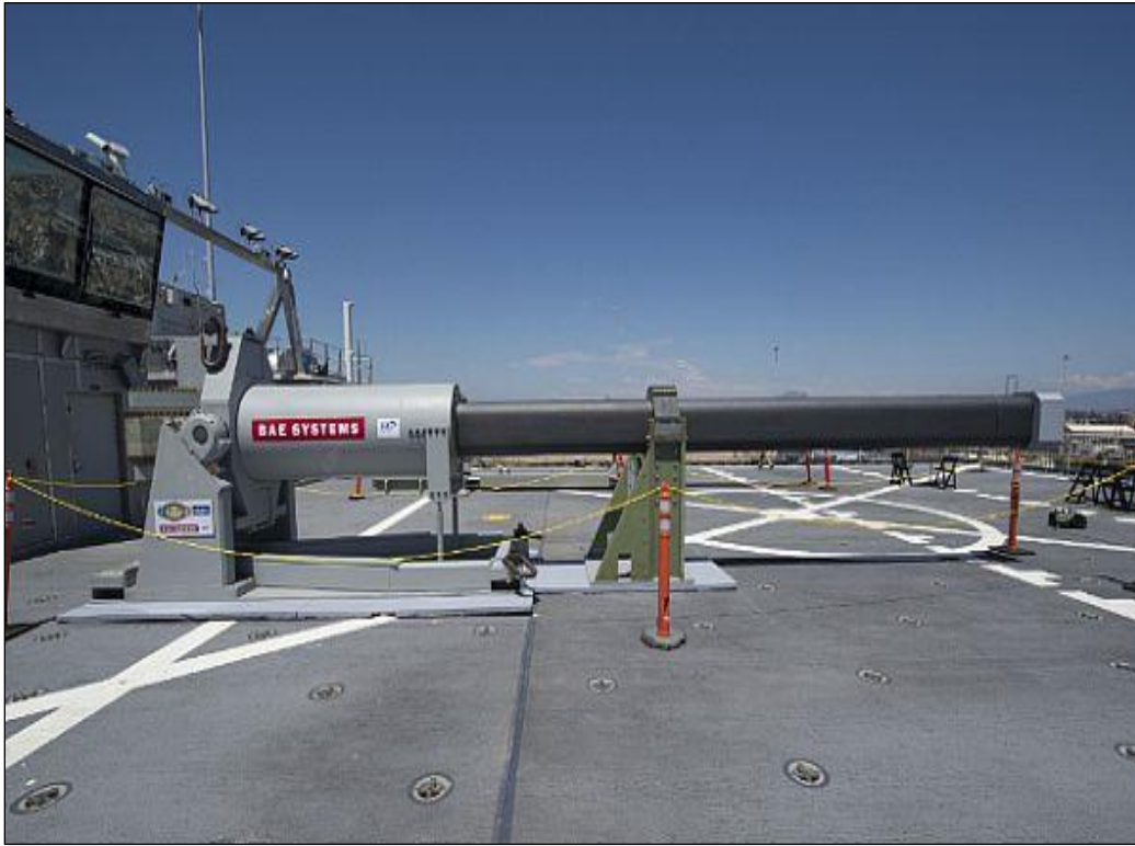
Figure 6. Industry-Built EMRG Prototype Demonstrator BAE prototype
