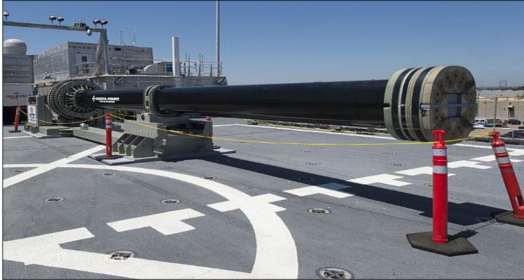
Figure 7. Industry-Built EMRG Prototype Demonstrator General Atomics prototype
