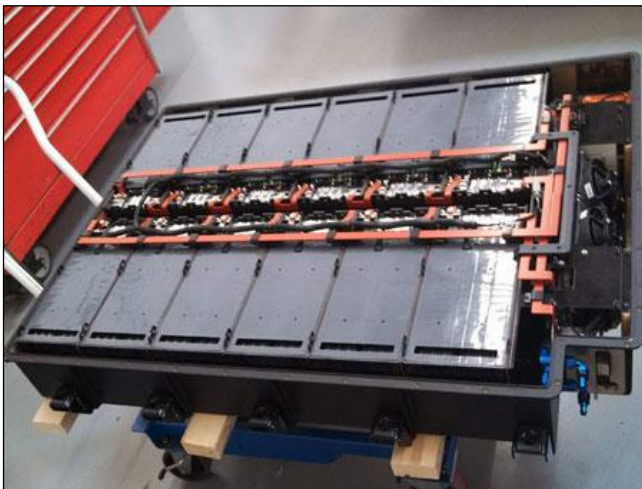
Figure 2. Inside an Electric Bus Battery Pack
