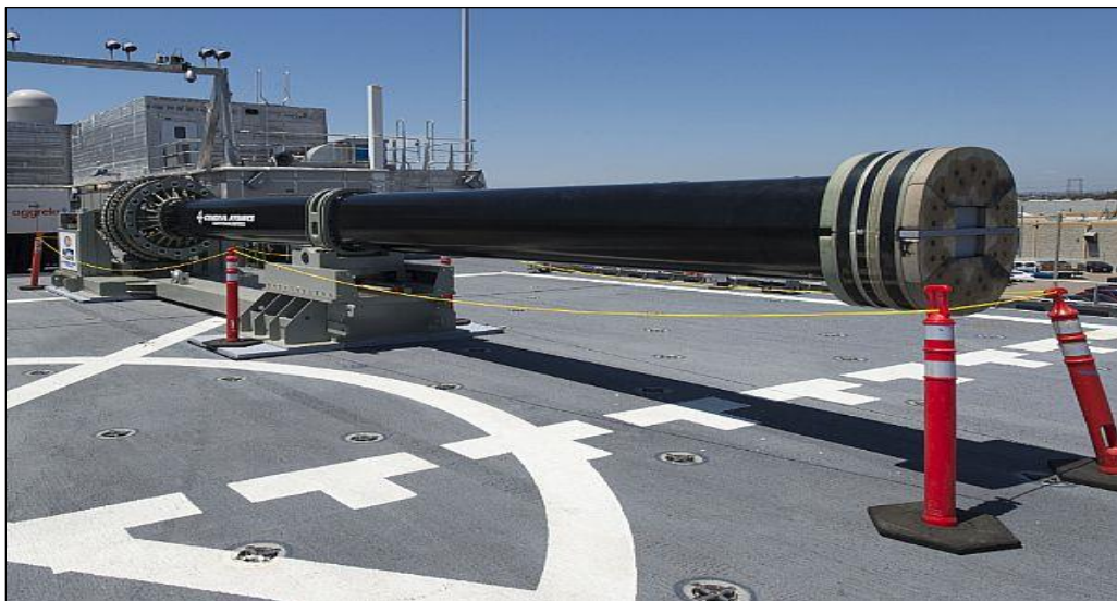
Figure 8. Industry-Built EMRG Prototype Demonstrator General Atomics prototype
