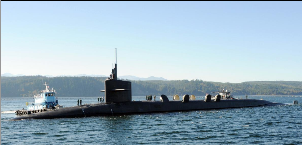
Figure I. Ohio (SSBN-726) Class SSBN With the hatches to some of its SLBM launch tubes open
