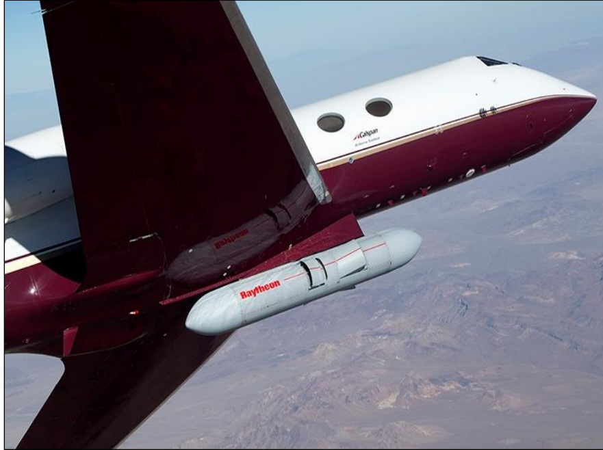
Figure 3. Next Generation Jammer Prototype Raytheon's NGJ Prototype mounted on a Gulfstream test jet
