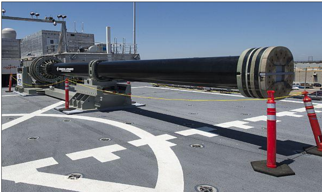
Figure 5. Industry-Built EMRG Prototype Demonstrator General Atomics prototype
