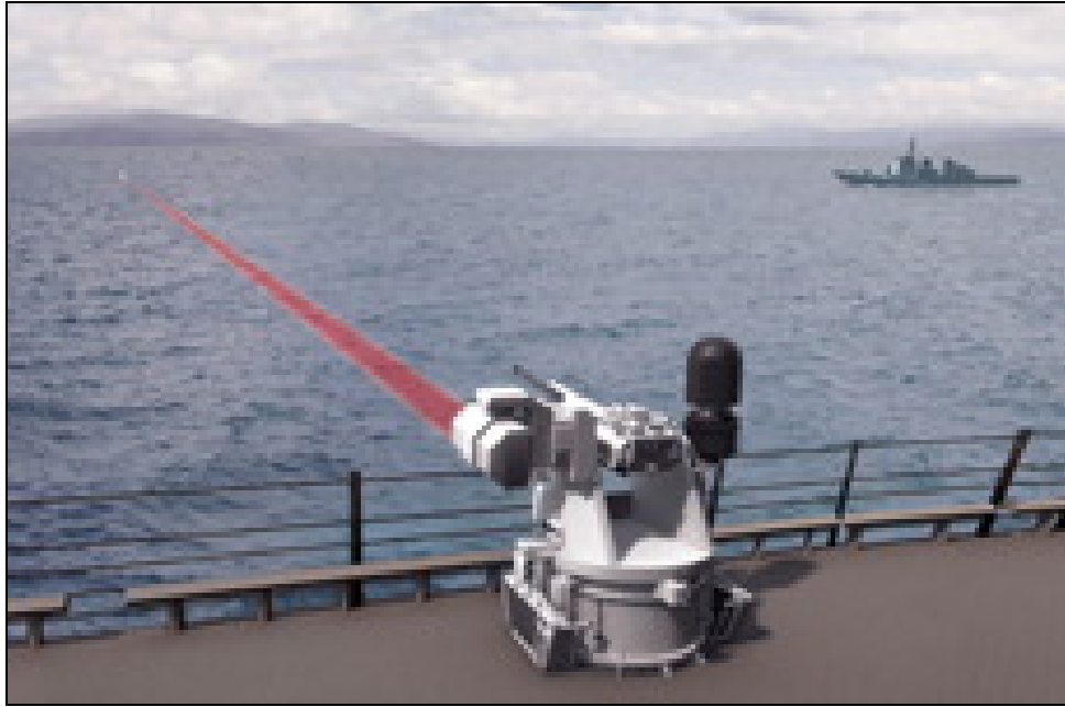
Figure D-1. Rendering of TLS Integrated on Mk 38 Machine Gun Mount
