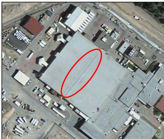
Figure 5. PF-4 Roof Showing Drag Strut
