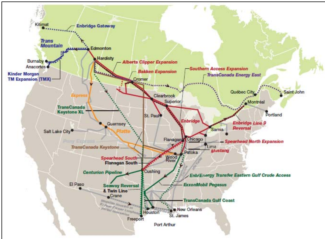
Figure 7. Oil Pipelines between Canada and the United States Existing (Solid Lines) and Proposed (Dashed Lines)
