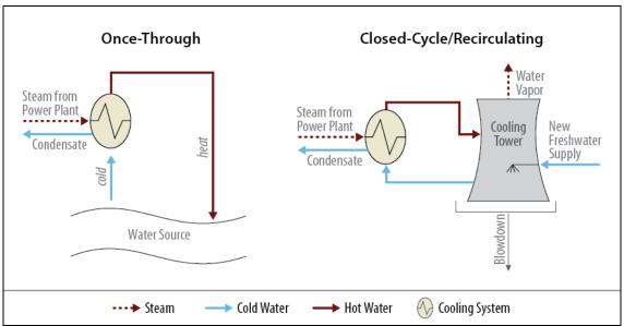
Figure 1. Once-Through and Closed-Cycle Wet Cooling System Designs
