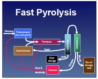
Figure 2. Biochar Production via Pyrolysis
