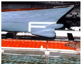
Figure D-I. Near-Surface Bow Bulb Design for DDG-51
