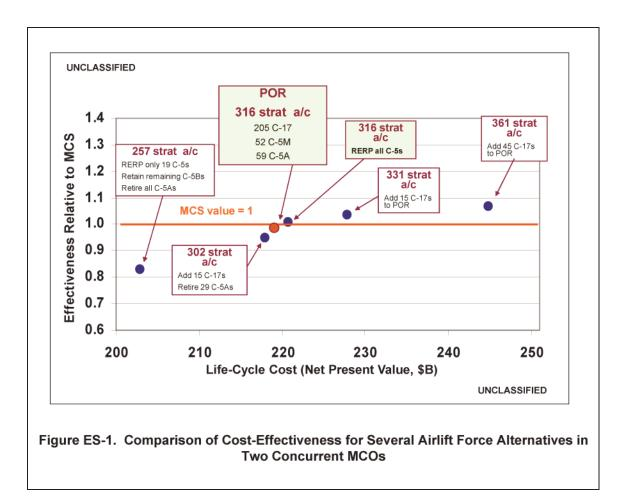
A small amount of additional capability could be achieved if all C-5s are converted through Reliability Enhancement and Re-engining Program (RERP) to C-5Ms. This alternative is at comparable life-cycle cost to that of the POR; near-term acquisition costs are almost repaid over time in later years by reduced operating and support (O&S) costs.
