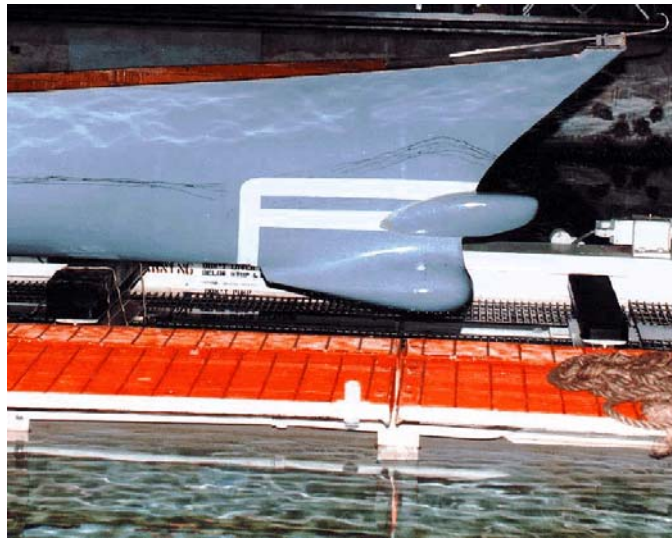
Figure D-1. Near-Surface Bow Bulb Design for DDG-51
