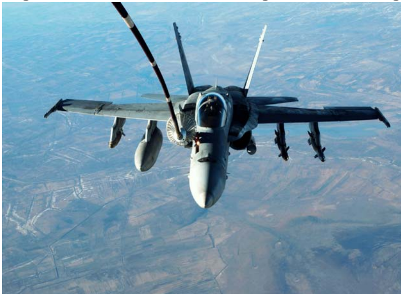
Figure 2. Photo of “Hose and Drogue” Air Refueling
