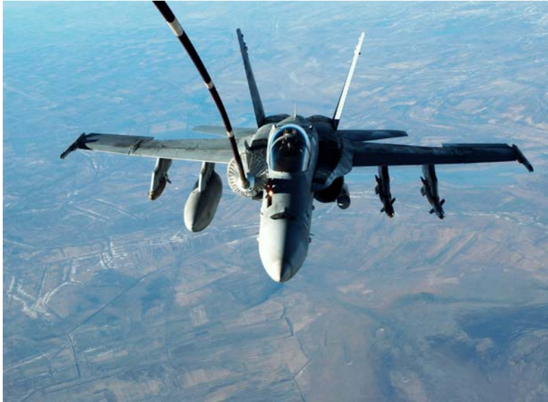
Figure 2. Photo of “Hose and Drogue” Air Refueling
