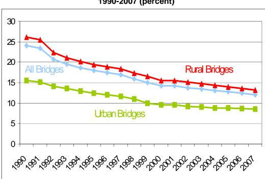
Figure 1. Structurally Deficient Bridges in the United States, 1990-2007 (percent)
