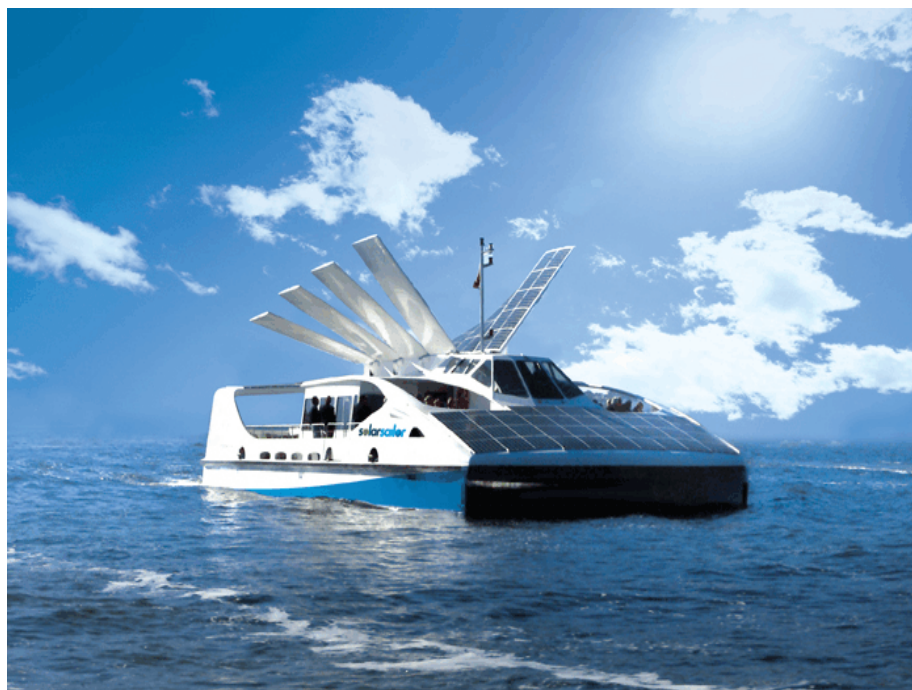
Figure 11. Solar Sailor Hybrid-Powered Ferry Boat
