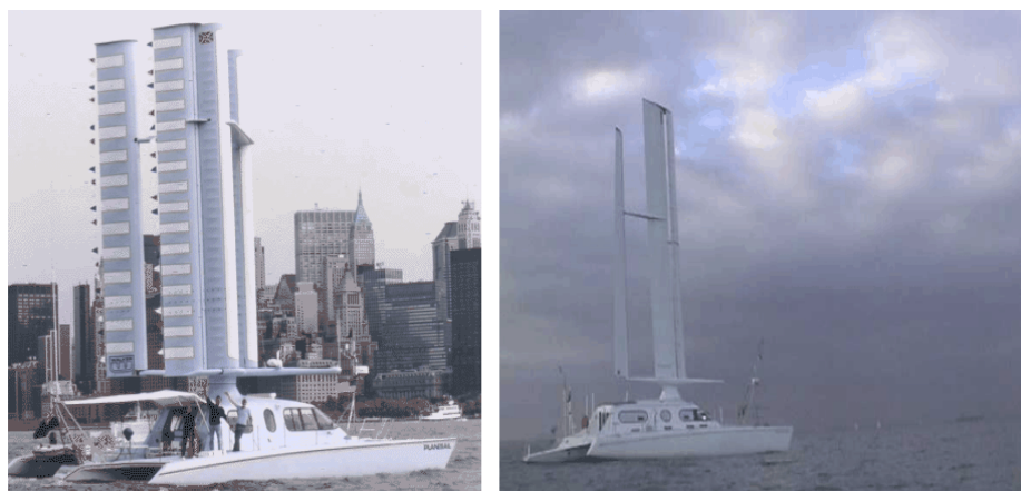
Figure 6. Pleasure Craft Equipped with Walker Wingsails
