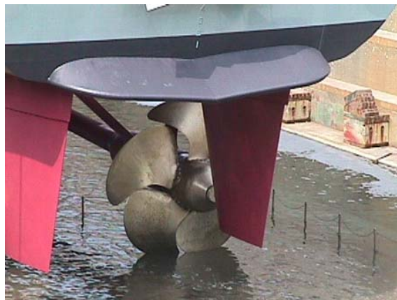
Figure 3. Stern Flap on DDG-51 Class Destroyer
