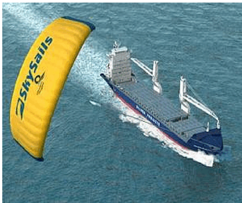
Figure 9. SkySails Concept Applied to Commercial Cargo Ship
